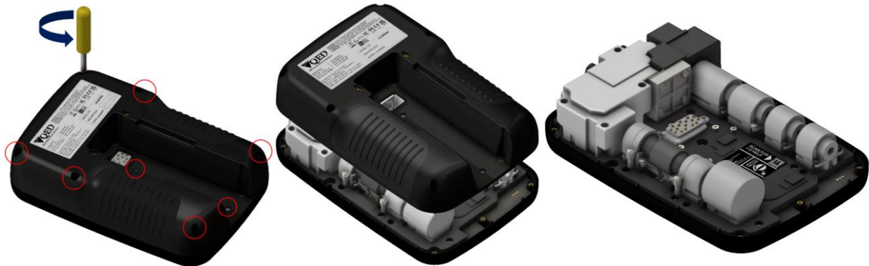
Figure 15 – Case Back Removal
