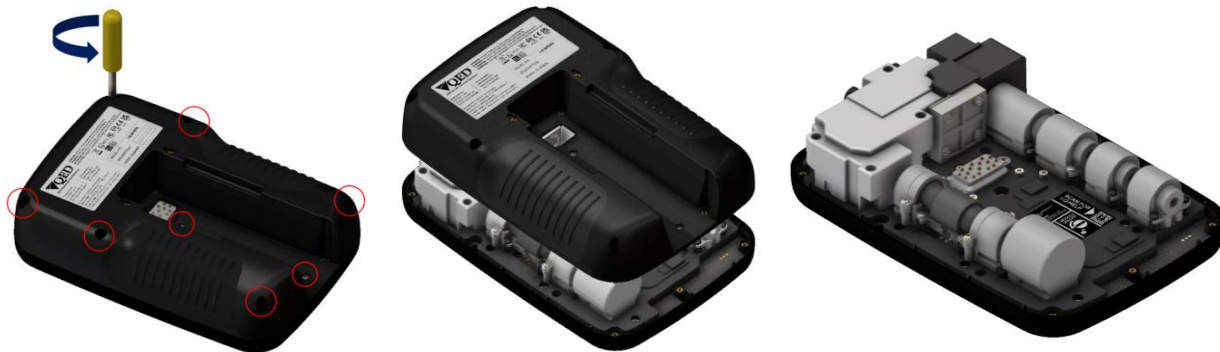
Figure 13 – Case Back Removal
